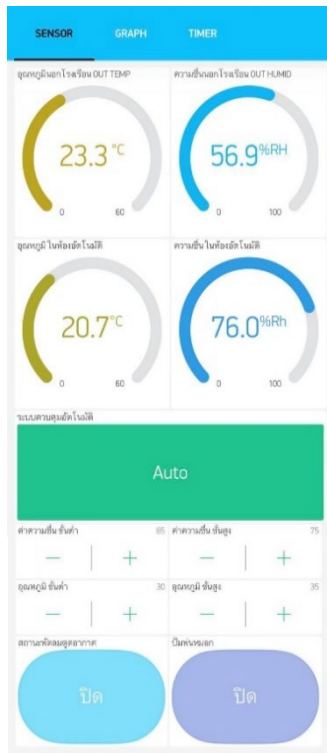
Fig. 10. The screen displays the oyster mushroom incubator's values.
